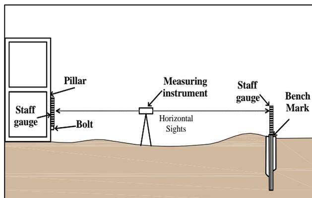
Figure 11 – Illustration of the geometric leveling method
