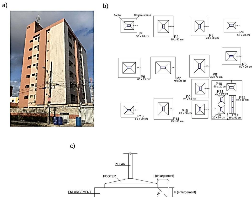
Figure 4 – a) Image of the Building b) Location of pillars and footings c) Detail of the footing enlargement
