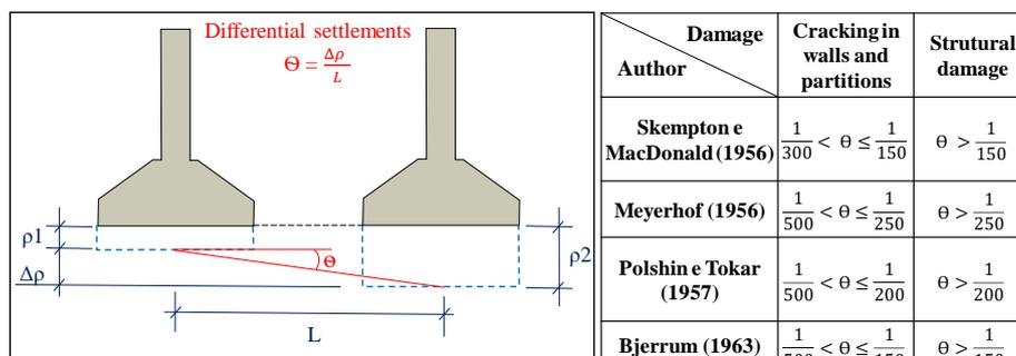
Figure 2- Threshold values of angular distortions  $\Delta\rho/L$  for structured buildings and armed bearing walls. Adapted from I.S.E. (1989) apud Velloso & Lopes (2011)
