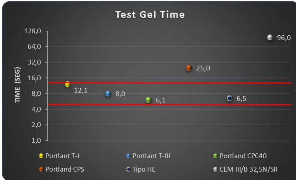
Figure 2 - The following graph shows the Evaluation of the Gel Formation Time in the backfill.
