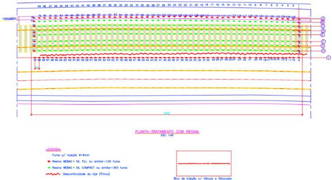
Figure 6 - Project for Injection Points – planning (initial)
