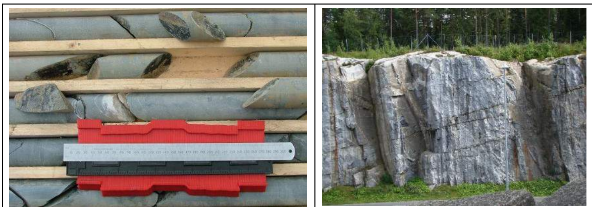
Figure 7 - An important part of Q-system application for NMT is of course core-logging and where possible, rock exposure logging. These are examples from the Bærum rail tunnel and from Follobanen. In the former roughness JRC was also logged to assist in pre-injection material selection based on interpretation of both Lugeon (and Q H2O ) and seismic refraction data.
